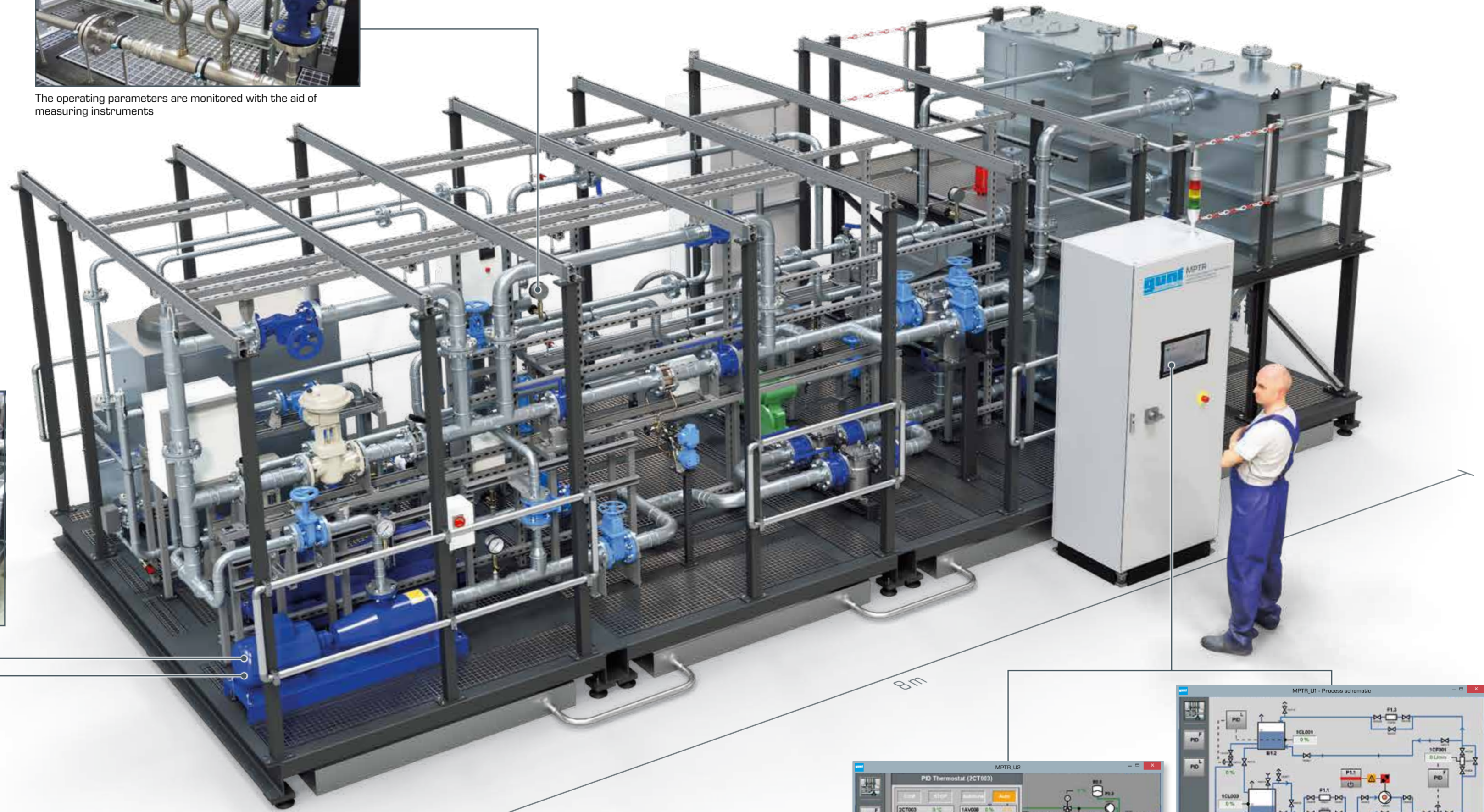
With different fittings different operating conditions can be set
